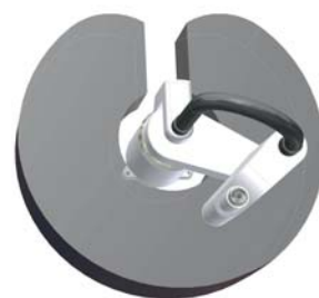
SCARA robots: kidney-shaped envelope with dead space
